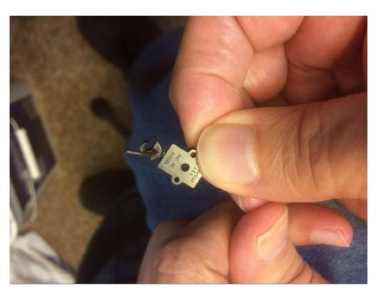
Now gently move the knuckle in the other direction. When the knuckle centers correctly, it's ready to be installed. If it does not center, rebuild.
