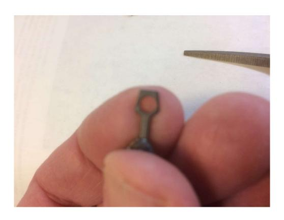
Check the face of the knuckle and gently remove any burrs on the seam.
